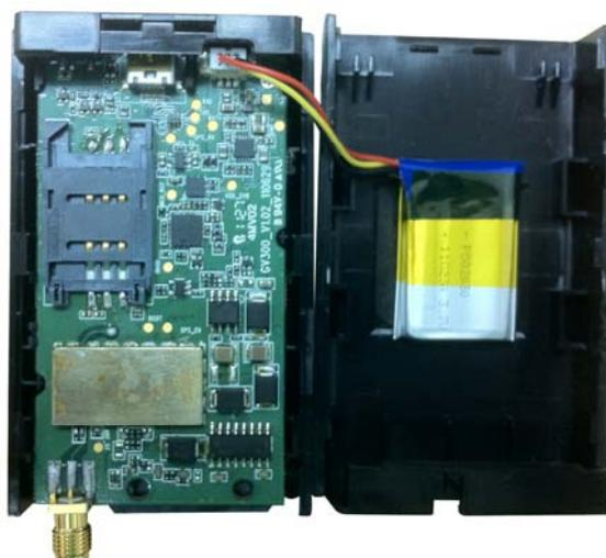
Figure 6. Backup Battery Installation
