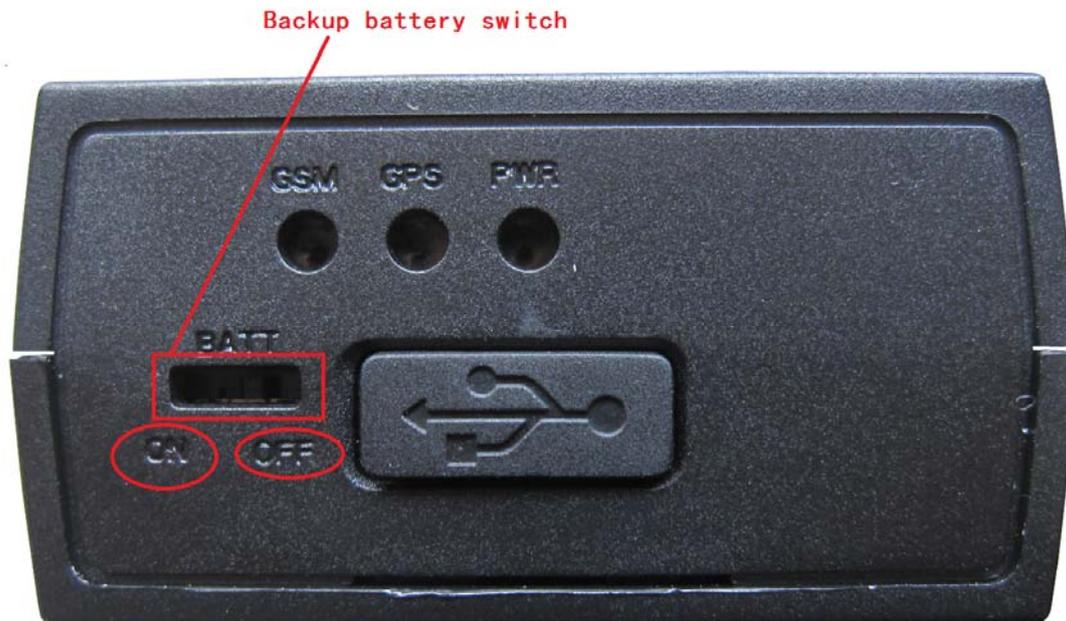
**Figure 7. Switch and ON/OFF position**
